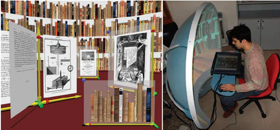
Figure A2. Mixed-reality library—In a project from the early 2000s of the Conservatoire national des arts et métiers (CNAM), Paris, using the VisonStation hardware by Elumens, a collection of physical books was digitized, rendered as facsimiles, and projected back into the physical space on a half-dome screen (Almeida et al. 2006). Note the axial arrangement of the pages on the left, reminiscent of old-fashioned museal equipment used for the display of individual folios of illuminations or engravings. (Reprinted by permission from Springer Nature Customer Service Centre GmbH: Springer, Technologies for E-Learning and Digital Entertainment by Z. Pan et al., CC-BY-NC 2006)
